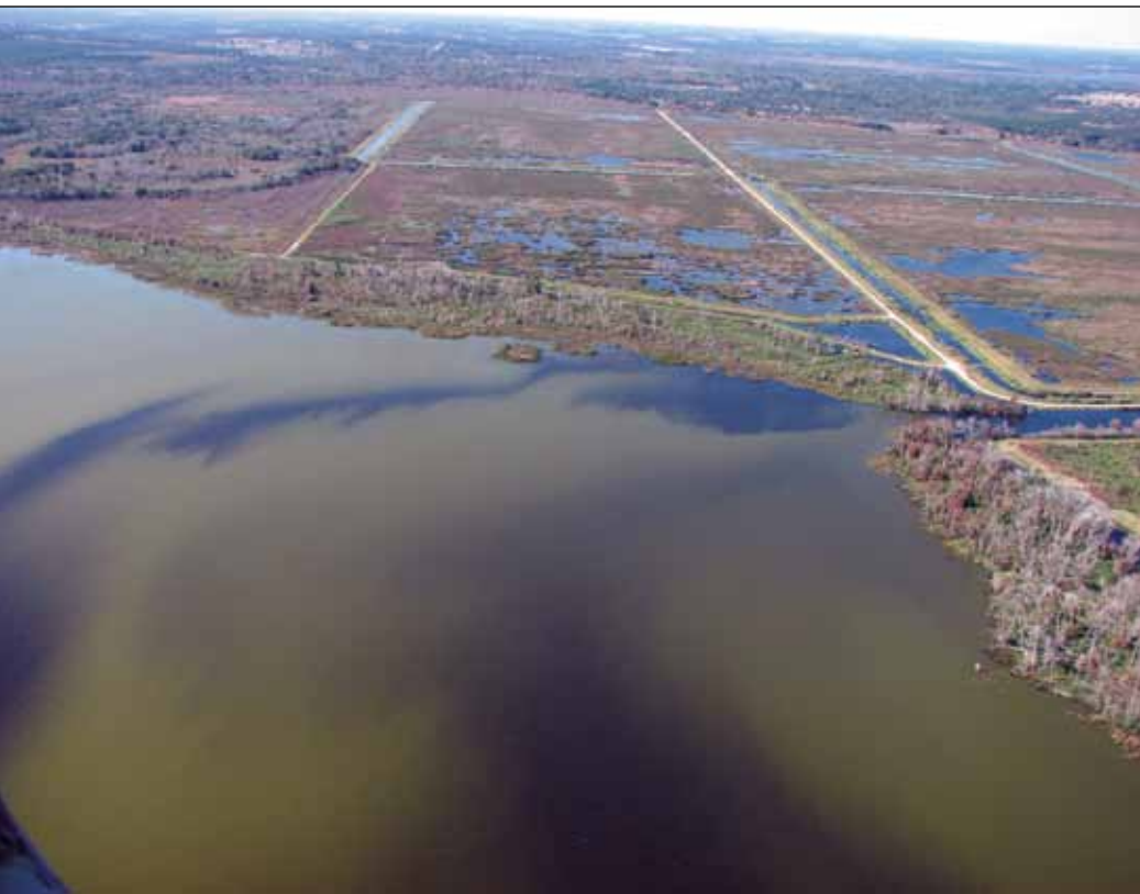
Figure 3. Plume of treated marsh flow-way water (clear water) being returned to Lake Apopka. Photo by Jim Peterson.
